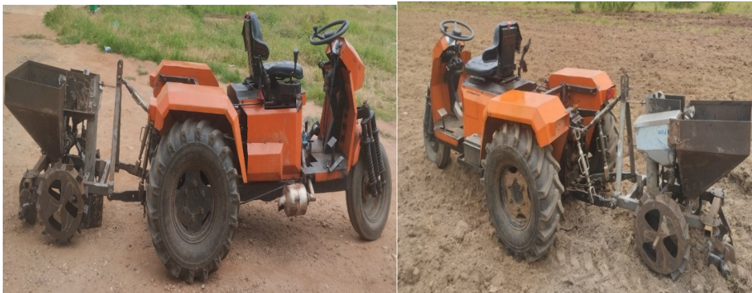
Plate 2: Calibration of developed tractor drawn single row Irish potato planter with fertilizer applicator
