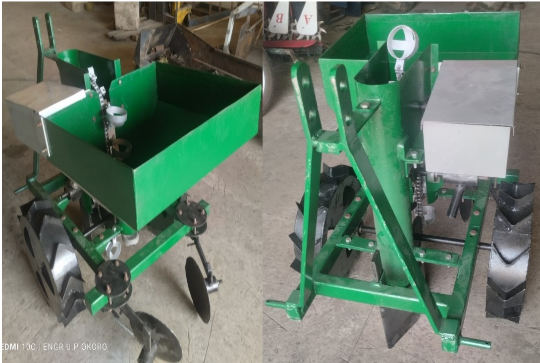
Plate 1: Pictorial view of the developed tractor-drawn single row Irish potato planter with fertilizer applicator.
