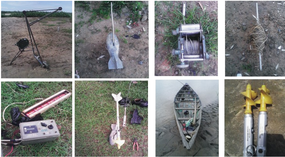
Plate 1: SK 100 suspended Derick, Sinker weight, Revolution counter, Fish Tail, Winch, Rod and thread, Boat and Braystock. Source: Fieldwork 2024
