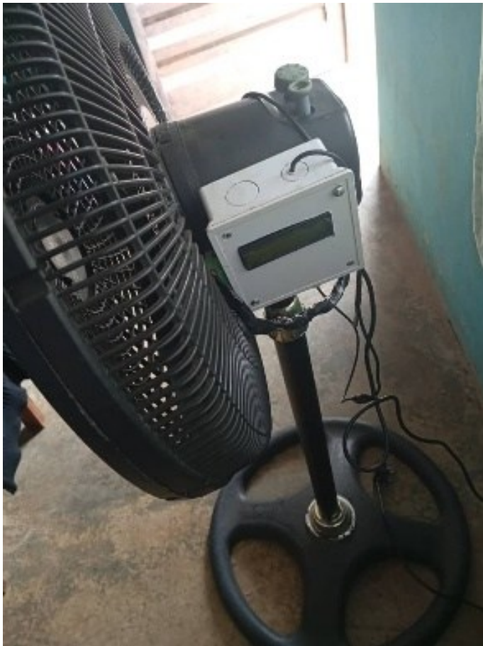
Figure 7: The developed system attached to an AC fan
